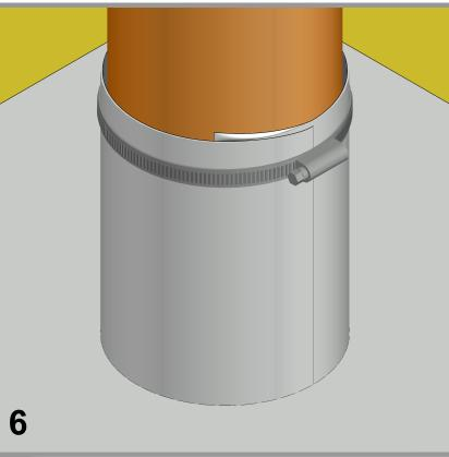
Secure upstand collar with a mechanical fastening.
