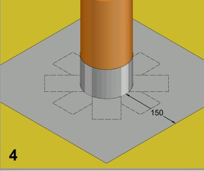
Cut central hole in a square of detailing strip. Square to extend minimum 150mm beyond base of pipe. Bond over horizontal strips and membrane.
