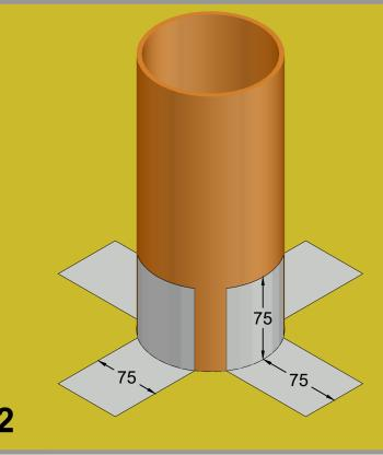
Bond 150mm x 75mm strips of VisqueenPro Detailing Strip as shown. Strips to be bonded 75mm onto pipe and 75mm onto membrane.
