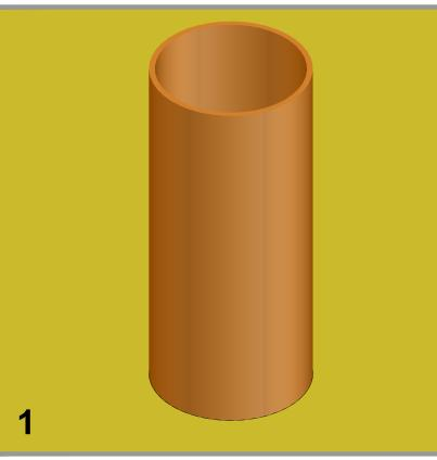
Ensure surface of pipe is clean and free from any contamination. Cut Visqueen High Performance Damp Proof Membrane to fit tight around base of pipe.
