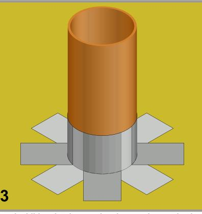
Bond additional strips overlapping previous strips by minimum 25mm.
